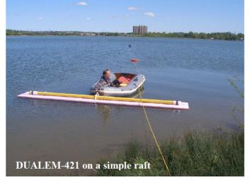
The DUALEM-421S has dual-geometry receivers at separations of 1-, 2- and 4-m from the transmitter, which provide six simultaneous depths of conductivity sounding, six simultaneous depths of susceptibility sounding, and detection of metal.
