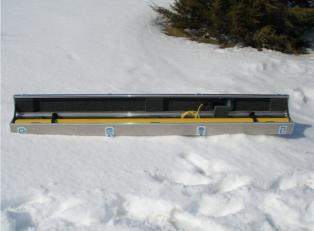
The DUALEM-2 has 2-m separation between its transmitter and dual receivers, so its dual depths of conductivity measurement are 1 m and 3 m (by the 70-% cumulative-sensitivity guideline). In-phase measurements sound magnetic susceptibility and detect metal.
