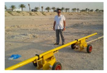
The DUALEM-642S has dual-geometry receivers at separations of 2-, 4- and 6-m from the transmitter, which provide six simultaneous depths of conductivity sounding, six simultaneous depths of susceptibility sounding, and detection of metal.
