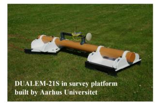
The DUALEM-21 has dual-geometry receivers at separations of 1- and 2-m from the transmitter, which provide four simultaneous depths of conductivity sounding, four simultaneous depths of susceptibility sounding, and detection of metal.
