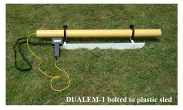
The DUALEM-1 has 1-m separation between its transmitter and dual receivers, so its dual depths of conductivity measurement are 0.5 m and 1.5 m (by the 70-% cumulative-sensitivity guideline). In-phase measurements sound magnetic susceptibility and detect metal.
