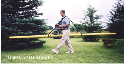
The DUALEM-4 has 4-m separation between its transmitter and dual receivers, so its dual depths of conductivity measurement are 2 m and 6 m (by the 70-% cumulativesensitivity standard). The DUALEM-4 depths of measurements are well suited to a variety of applications in agriculture, geotechnics and hydrology. For metal detection,
